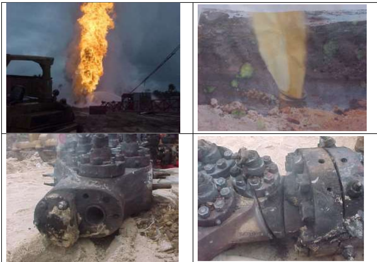
Figure 8.8: Oil blowout on a production well onshore Nigeria, 2006.
