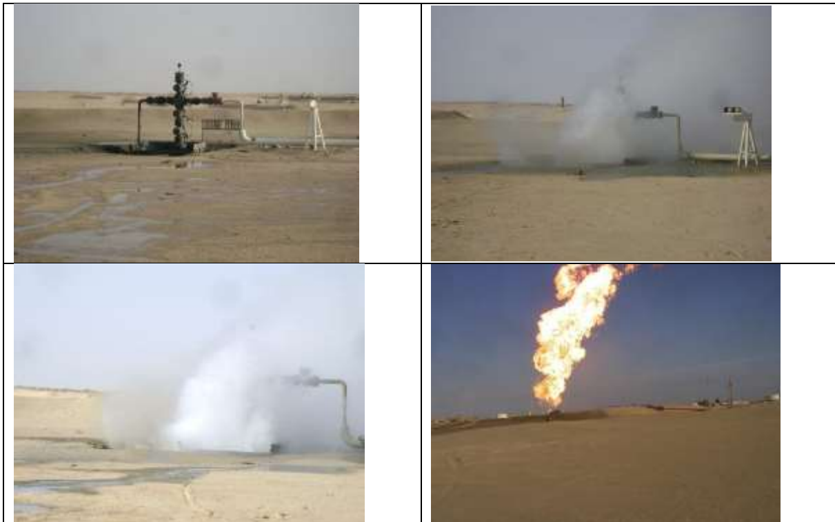
Figure 8.4: Gas blowout Libya 2011
