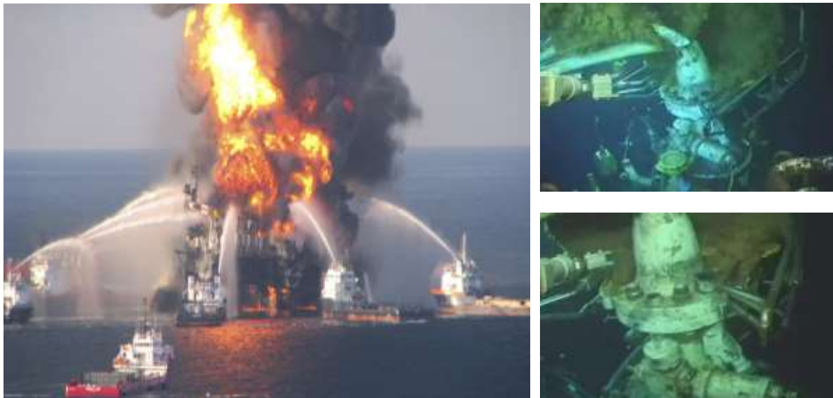
Figure 8.5: Macondo 2010, Initial fire-fighting and flow through subsea BOP
